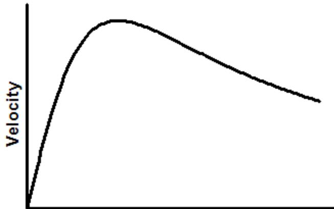
$$v = \frac{V_{MAX} S \left( 1 + a \frac{S}{K_{si}} \right)}{K_s + S \left( 1 + \frac{S}{K_{si}} \right)}$$
